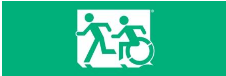
Figure 36: Proposed 'Running Man' and 'Accessible Means of Egress Icon' Exit Sign
